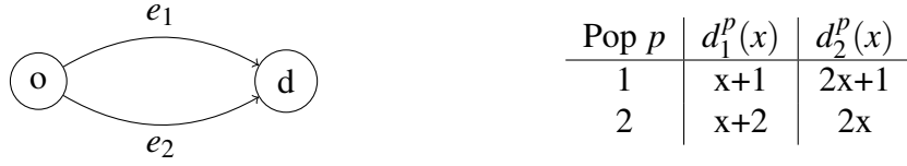
Fig. 2.5 Since the delay functions are in the form d_e^p(f_e^{agg}) = d_e(f_e^{agg}) + t_e^p , this routing game admits a potential function despite being heterogeneous.
